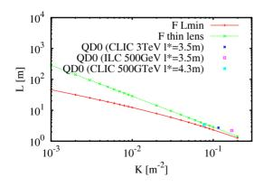
Figure 1: F as a function of magnet gradient. L is included for reference.
