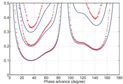
Figure 2: Solid blue and dotted red curves show  $\sqrt{\langle \psi_0 \rangle}$ and  $\sqrt{\langle \Psi_0 \rangle}$ , respectively, as functions of the cell phase advance. The measurement errors are beam size independent and are normalized to coincide with the relative errors of 10%, 20% and 30% for  $\mu_p = 45^{\circ}$  (from lower to upper pairs of curves).
