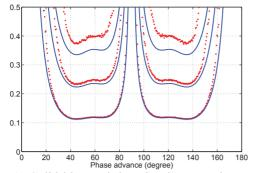
Figure 1: Solid blue and dotted red curves show  $\sqrt{\langle \psi_0 \rangle}$ and  $\sqrt{\langle \Psi_0 \rangle}$ , respectively, as functions of the cell phase advance. The measurement errors are relative and are equal to 10%, 20% and 30% (from lower to upper pairs of curves).
