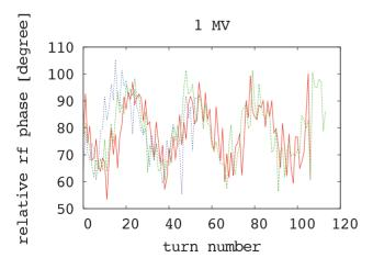
Figure 6: Synchrotron oscillations in EMMA.
