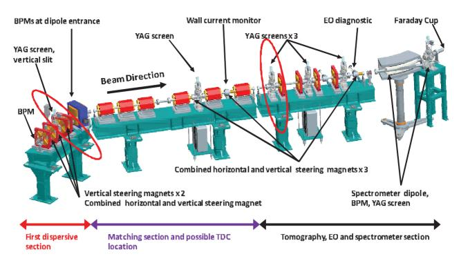
Figure 1: EMMA extraction and diagnostics line (YAG screens 01 and 03, used later for Figs. 4 and 5 are circled in red).
