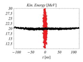
Figure 3: Longitudinal phase space rotation as required by the PRISM project (red before rotation, black after).
