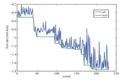
Figure 5: Beam loss rate of all evaluated solutions.
