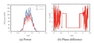
Figure 4: S2E simulations for circular polarization FEL with high power output, *left*: FEL powers in  $E_x$  and  $E_y$  direction, *right*: The phase difference of  $E_x$  and  $E_y$ .
