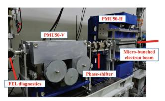
Figure 6: The installed CPU with phase-shifter at SDUV-FEL.
