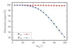
Figure 3: Phase error effect to the FEL polarization in EPU
