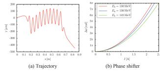
Figure 7: Trajectory and shifted phase from magnetic measured result of PMU50-V and phase-shifter, *left*: calculated electron trajectory in PMU50-V at the gap of 14 mm, *right*: the shifted phases at different stimulated currents.
