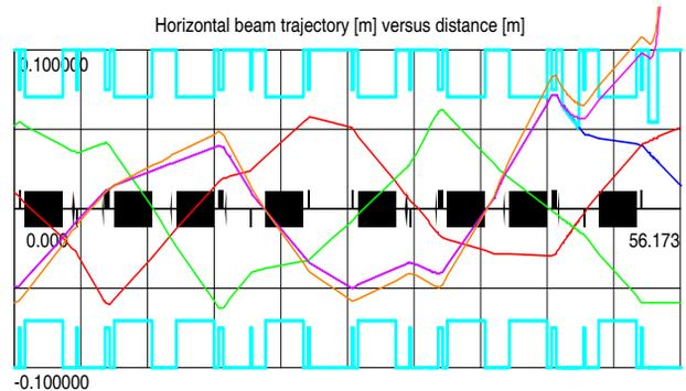
Figure 7: The trajectory of the last three turns before extraction and the extracted segment between ES and MS.
