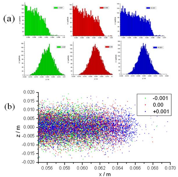
Figure 6: Extracted particle distribution at the entrance of the ES. From the top: horizontal direction, vertical direction, real space with a coordinate x-z.
