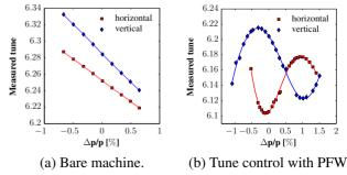
Figure 1: Influence of auxiliary coils on the linearity of the machine.
