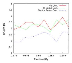
Figure 7: Comparison of dynamic aperture w/o skew sextupole corrections. Beam-beam effect is included.
