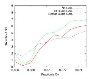
Figure 6: Comparison of dynamic aperture w/o skew sextupole corrections. Beam-beam effect is excluded.
