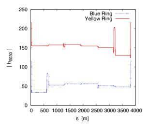
Figure 3:  $3Q_y$  RDTs in the Blue and Yellow rings without correction.
