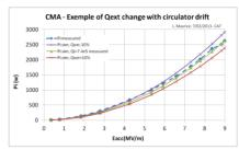
Figure 11: Effect of the circulator thermal drift on the cavity  $Q_{\text{ext}}$ .
