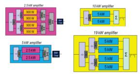
Figure 2: Amplifier architecture.
