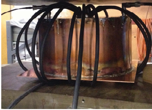
Figure 3: Re-entrant test cavity made of copper with toroidal coil for 2-directional magnetic bias testing.
