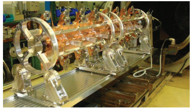
Figure 4: Accelerating structure mock-up after the last assembly operation (EBW).
