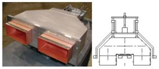
Figure 4: Photograph of a U-bend phase shifter with fingerstock to contact mating waveguide and drawing showing interior construction and pressure feed-throughs.
