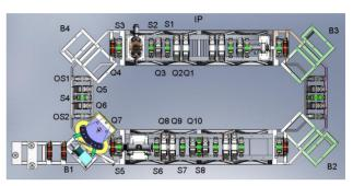
Figure 2: NESTOR storage ring lattice layout. B1-B4 are dipole magnets with combined focusing function, Q1-Q10 are quadrupole magnets, S1-S7 are sextupole magnets, OS1-OS2 are octupole magnets combined with sextupole magnets.
