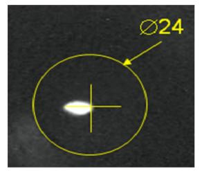
Figure 7: Electron beam shape behind the second bending magnet of the transporation channel the (9, Fig. 1).
