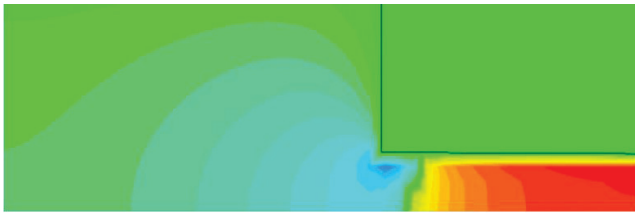
Figure 2: Contour plot of longitudinal electric field across one quarter of the periodic, side-open structure for the lowest confined mode at \sim 316 GHz.
