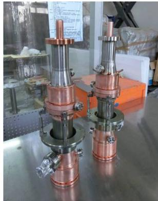
Figure 4: Two fabricated IHEP 1.3GHz input couplers.
