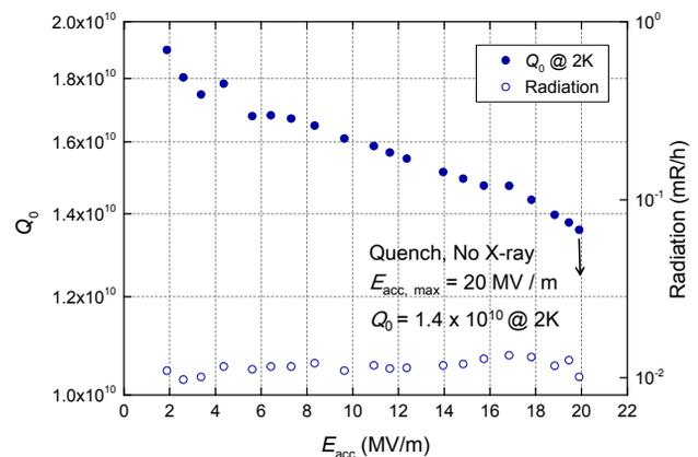
Figure 2: Test result of the IHEP-02 LL LG cavity.
