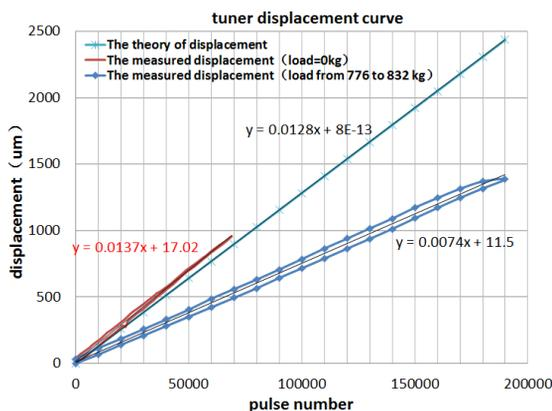
Figure 9: Motor tuner test curve.
