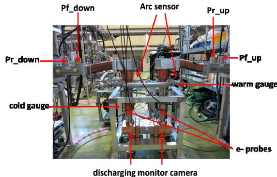
Figure 5: High power test stand.
