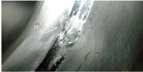
Figure 3: Weld plug machined and positioned ready for welding.
