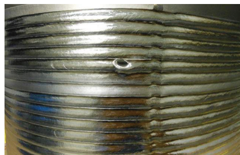
Figure 2: Baseline weld tests with original parameters, a hole is visible in the center of the image.
