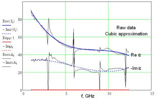
Figure 2: RF parameters of a SiC sample measured at 77 K. Details are described in [7,8]
