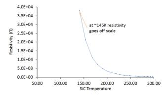
Figure 4: DC conductivity measured during a thermocycle of the SiC ring before brazing, indicating a strong increase with lowering temperatures.
