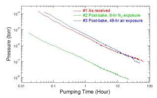
Figure 6: Pumpdown and outgassing test of the shrink-fit assembly. Besides the porous behaviour of the SiC no signs of gas burgs from the shrink-fit could be observed.
