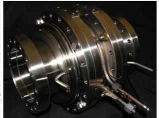
Figure 3: Picture of the HOM beamline absorber prior to installation in the HTC.
