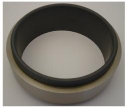
Figure 5: Silicon carbide ring shrink-fitted into a titanium grade 5 cylinder. After 2 thermo-cycles to 77 K neither visible damage nor loosening was observed.
