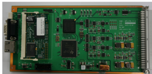
Figure 1: DSP Board that includes DSP, FPGA, ADCs and the other components.
