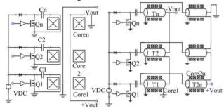
Figure 4. Simplified schematics of an inductive adder on the left, and a transmission line adder on the right.
