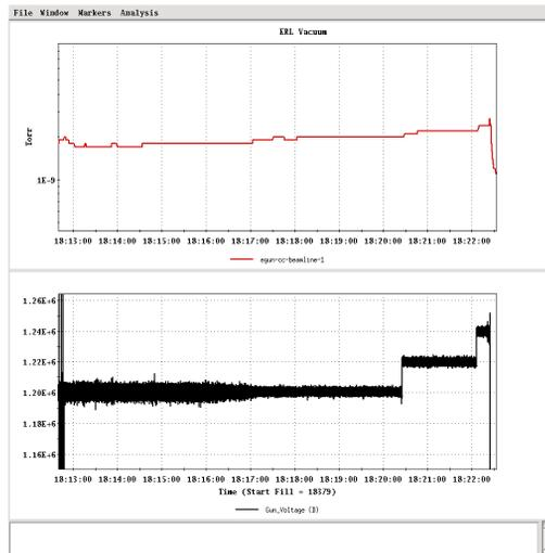
Figure 1: Beam-line vacuum (red) and gun voltage (black) during 1.2 MV CW operation of 704 MHz SRF gun at BNL.
