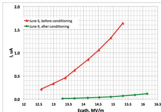
Figure 7: Dark current measured at faraday cup vs field at the cathode, before (red) and after (green) conditioning. Reduction is 25 times.
