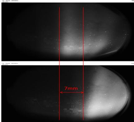
Figure 5: Dark current image taken at beam profile monitor during energy measurement at gun voltage settings 1.2 MV. Corrector current top 0.5 A, bottom 1 A. 7mm shift due to 0.5 A corrector change corresponds to beam energy of 1.2 MeV.
