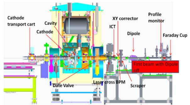
Figure 3: Schematic layout of the SRF injector at BNL R&D ERL.
