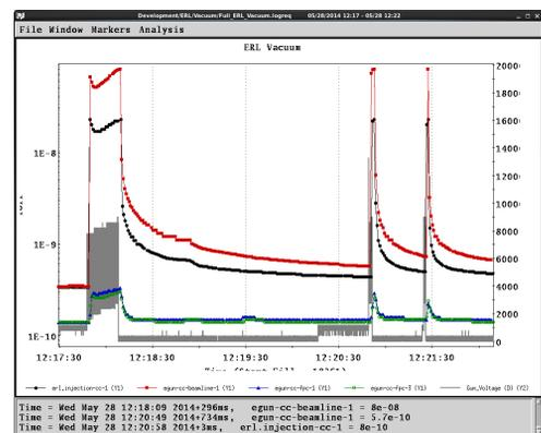
Figure 4: Vacuum spikes as observed during initial start of SRF gun operation with cathode inserted: gray color is gun voltage, other colors vacuum in different section of beam line.
