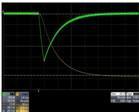
Figure 6: Faraday cup signal (green -225mV peak) due to dark current and its integral (yellow 28 mVsec).
