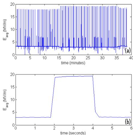
Figure 2: 5 cell cavity performance during horizontal test. Pulses are 2 seconds long with a 30 second interval.
