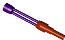
Figure 2: The FLUKA simulation model of the Tungsten collimator from the COMET cyclotron.
