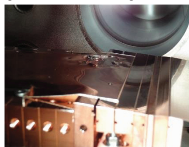
Figure 3: Damage found on the cover foil of the short gap in-vacuum undulator SGU#17.
