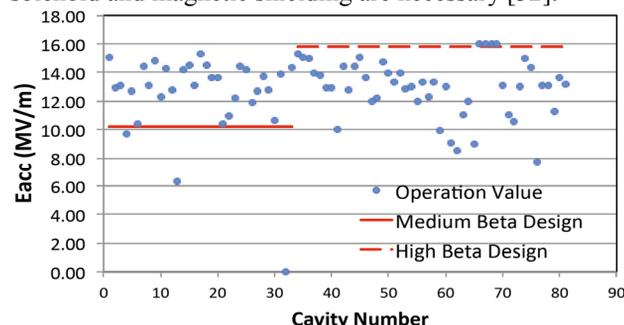
Figure 3: Accelerating gradients of the 81 SNS  $\beta=0.61$  (medium) and  $\beta=0.81$  (high) cavities in 23 cryomodules.
