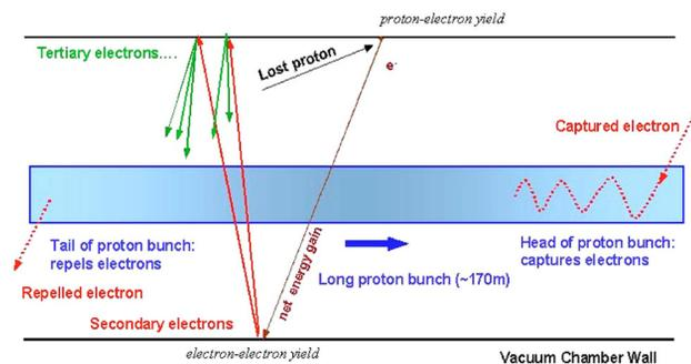
Figure 12: Beam-induced electron multipacting at the trailing edge of a long proton bunch [6].
