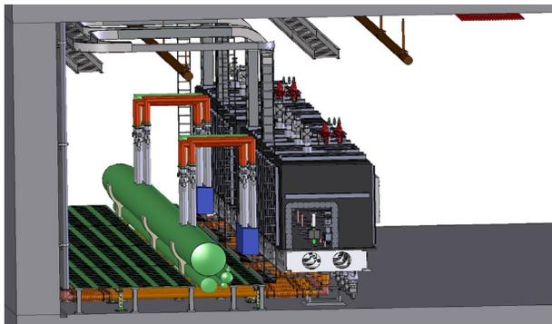
Figure 4: FRIB cryomodule with U-tube connections.
