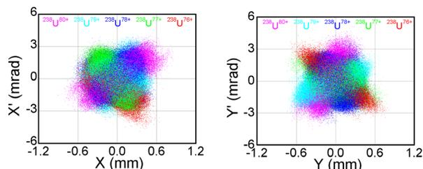
Figure 11: Five charge states of the uranium beam designed to overlap at the FRIB target.
