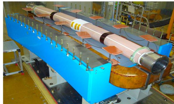
Figure 9: J-PARC RCS dipole and vacuum chamber.
