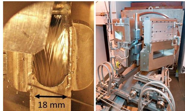
Figure 8: (left) SARAF’s liquid lithium target under test [48] and ISIS spallation target station 2 [46].
