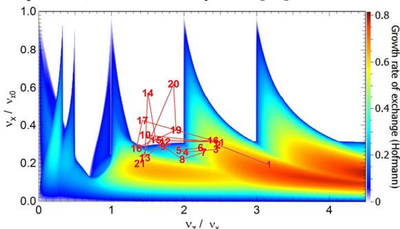
Figure 10: Tune footprint along the four IFMIF cryomodules superimposed to the Hofmann chart [60].
