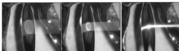
Figure 6: Liquid lithium film intercepting a proton beam of ~ 60 kV for beam power survival test [41].
