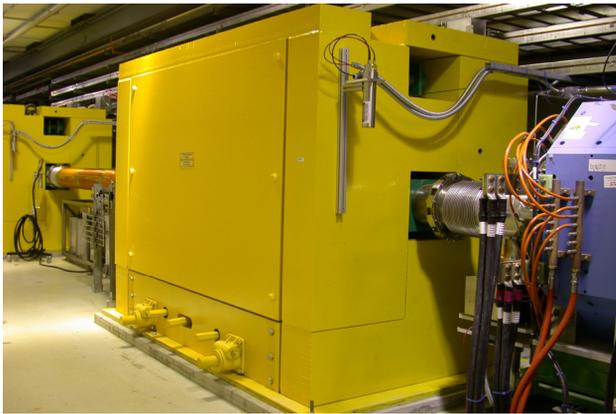
Figure 7: SNS two-stage, multi-layered collimators, each designed to withstand 10 kW protons at 1 GeV.
