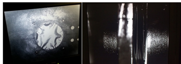
Figure 17: The stripping foil inside the solenoid seen from the diagnostics chamber in front of the solenoid (left) and via the non-destructive lateral view port pointing toward the solenoid centre (right).
