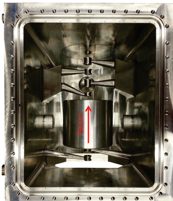
Figure 1: Top view of the FRANZ IH-cavity. Between entrance and quadrupol triplet (aluminum dummy) are three gaps and between lens and exit are five gaps. On the side of the triplet the static frequency plungers (aluminum dummy) are shown.
