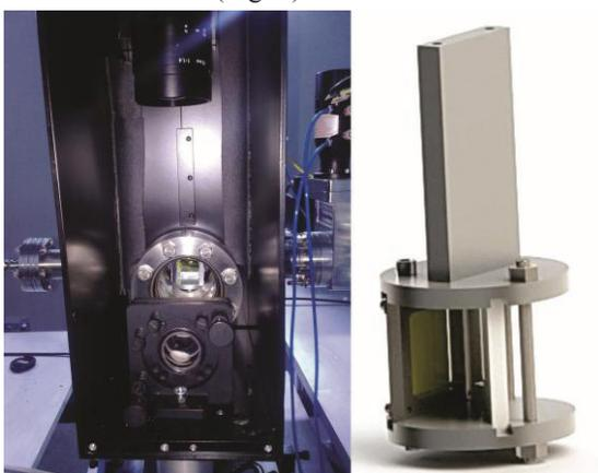
Figure 4: Optical black box and YAG:Ce holder.
