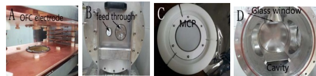
Figure 6: Picture of IPM components (a) inside view of the OFC electrodes (b) external view of the chamber (c) a MCP + Screen (d) inside view of the empty chamber.
