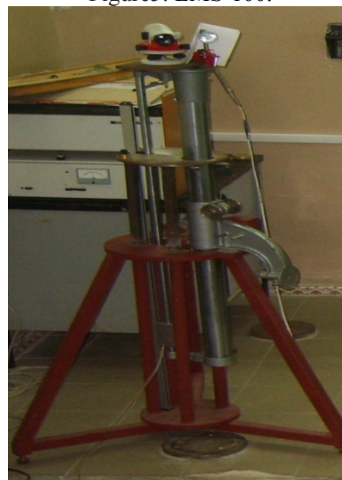
Figure 6: Level of Leica company, on a portable tripod with the measuring system LIR- 7.
