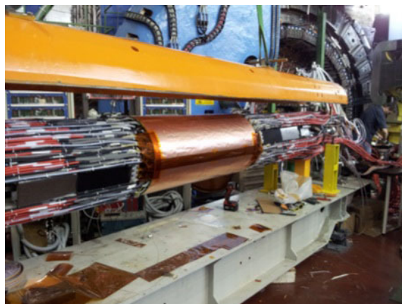
Figure 2: The DAΦNE IR with the new detector layers ready to be inserted in KLOE-2.
