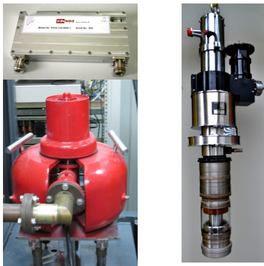
Figure 4: The RF amplifiers: 2W (left top), 10 KW TH 2436 (left bottom) and 7 MW K211 klystrons (right).
