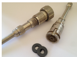
Figure 1: Picture of coaxial sample holder used for reflection and transmission measurements.
