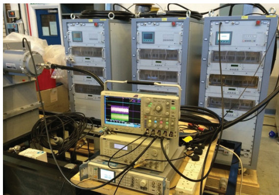
Figure 7: Setup for 8kW FETS amplifier tests.
