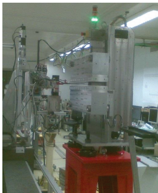
Figure 1: The undulator on the Hasylab magnetic test bench.
