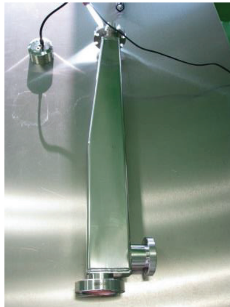
Figure 4: Inlet/outlet chamber for electron beam vacuum system.
