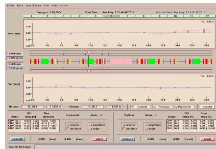
Figure 1: The selected bump and correctors at bending magnet photon source in section 6.
