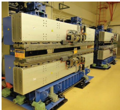
Figure 1: Two EPU48s of TPS phase-I beamline project.
