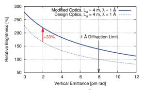
Figure 4: Brightness increase (at 1 Å) from the modified optics compared to the design optics for different settings of emittance coupling in the MAX IV 3 GeV storage ring.
