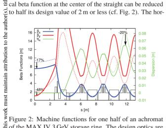
Figure 2: Machine functions for one half of an achromat of the MAX IV 3 GeV storage ring. The design optics are indicated in dashed lines, while the solid lines indicate one possible modified optics.
