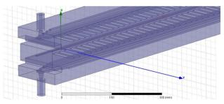
Figure 1: Model of the slotted kicker. The model shows one end of the slotted kicker, with the other end being a mirror image. The model contains the power ports, transmission lines, waveguides, beam pipe, and slotted interfaces. The *x*-axis is physical vertical direction of the beam motion.
