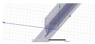
Figure 3: Slotted kicker with longitudinal ports and a linear taper from the cylindrical coax to the rectangular transmission line.
