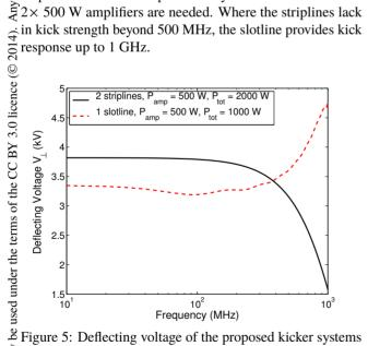
$\stackrel{\scriptscriptstyle {\mathcal{B}}}{\rightarrow}$  Figure 5: Deflecting voltage of the proposed kicker systems  $\frac{3}{2}$  in the SPS. Note that the stripline array requires  $4 \times 500$  W TUPRI087 06 Ins
