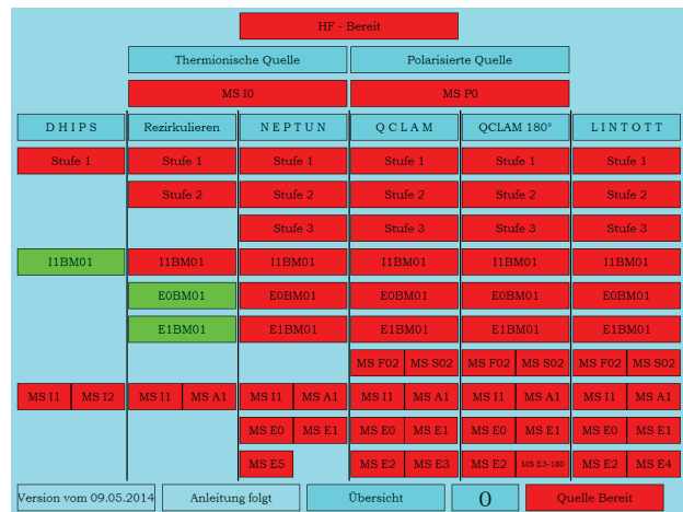
Figure 4: On this screen the operator can choose the electron source as well as the beam mode. The corresponding column shows the superior conditions which need to be fulfilled for the operation.
