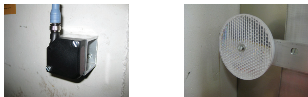
(d) The combined emitter and acceptor element of the light barrier. (e) The reflector mirrors the signal coming from the emitter back to the acceptor.
