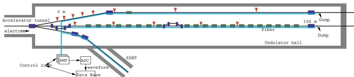
Figure 1: Schematic view of the Cherenkov beam loss monitor system in SACLA. Aqua blue lines indicate the optical fibres for the beam loss monitors. Green boxes, blue boxes and red triangles indicate the undulators, the bending magnets and the screen monitors.
