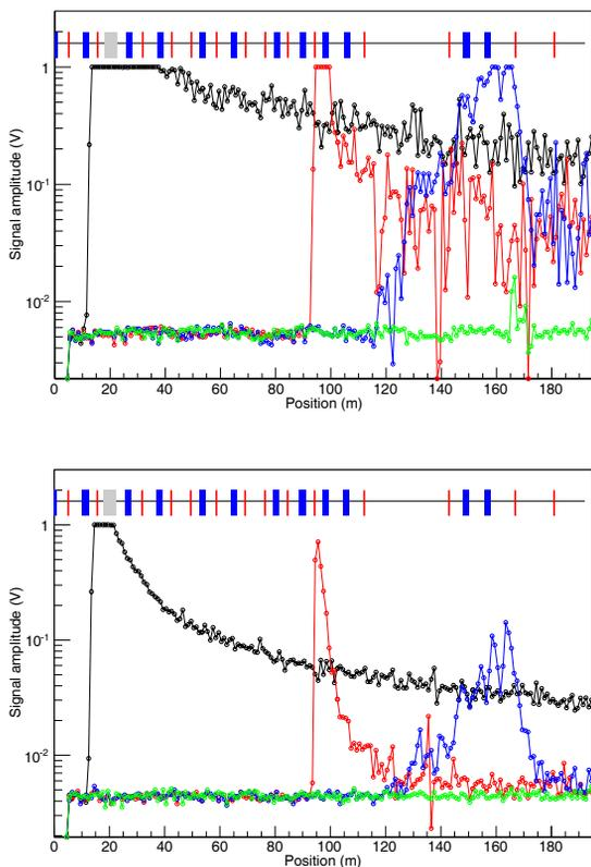
Figure 4: The signals from the high gain (upper) and low gain beam loss monitor (lower) during the commissioning of XSBT. Blue boxes and red lines indicate the bending magnets, the screen monitors respectively. The grey box indicates the shield wall between the undulator hall and XSBT tunnel. Black and red line shows the signal of the beam loss monitor with inserting the screen monitor. Blue and green line shows the beam loss in the progress of the accelerator tuning.
