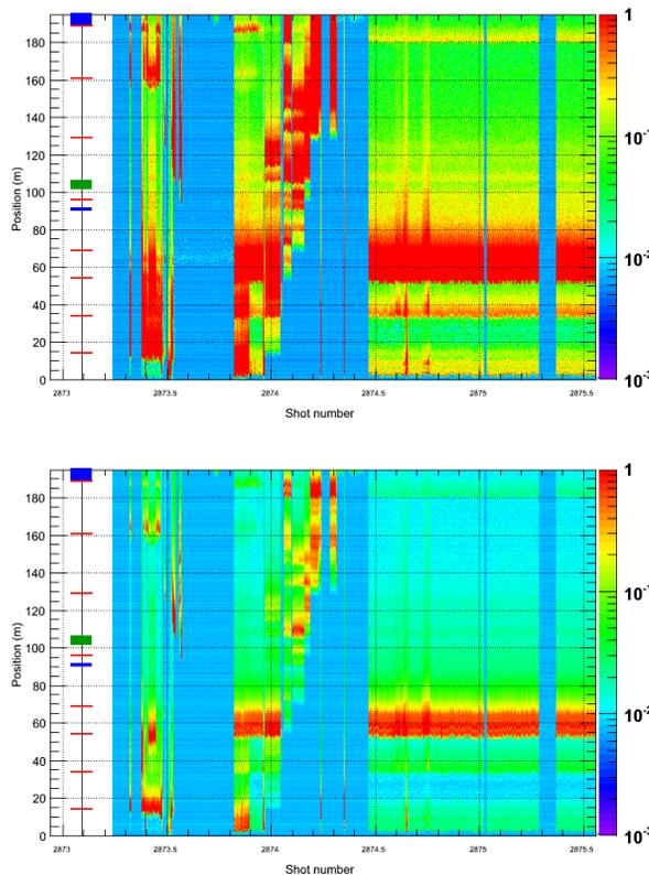
Figure 2: The signal from the high gain (upper) and low gain beam loss monitor (lower) in accelerator tuning. The magnitude of the monitor signal (color scale in voltage) as a function of the shot number (horizontal axis) and the position of the beam loss (vertical axis). Red line, blue box and green box indicate the screen monitor, the undulator and the bending magnet.
