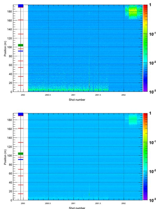
Figure 3: Beam loss in halo monitor experiment. The magnitude of the monitor signal (color scale in voltage) as a function of the shot number (horizontal axis) and the position of the beam loss (vertical axis).
