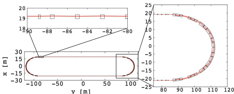
Figure 4: Layout of the ring with magnified cells in the production straight and in the arc together with muon closed orbits. The racetrack shape of the ring is dictated by the need of a high neutrino production efficiency.
