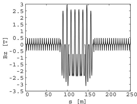
Figure 3: Vertical magnetic field on the median plane for the max momentum muon in the nuSTORM RFFAG ring.
