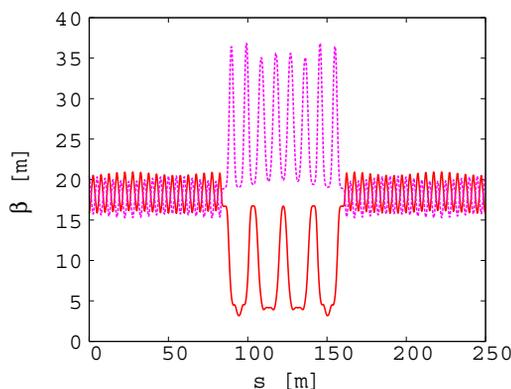
Figure 1: Horizontal (red line) and vertical (pink one) betatron functions in the half of nuSTORM RFFAG ring.
