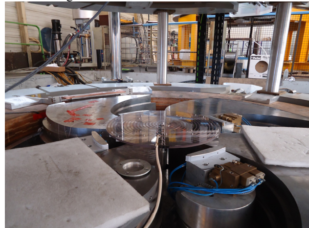
Figure 6: B_r mapping system for the C230 PAP125 cyclotron.
