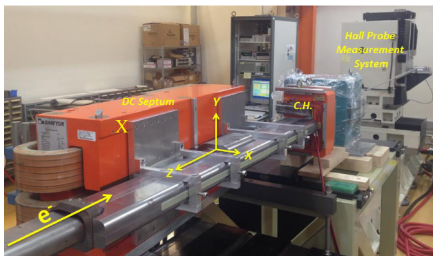
Figure 8: Layout of the Hall-probe measurement system .
