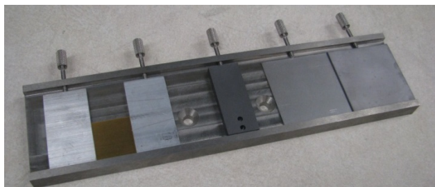
Figure 2: Target holder with Au, C, Fe, and Ta targets from left. Aluminium plates are used to hold Au target.
