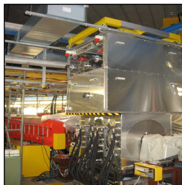
Figure 1: The first of three new MA acceleration cavities installed and commissioned in SIS18.
