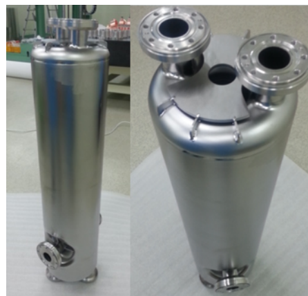
Figure 4: Quarter wave resonator after final electron beam welding.
