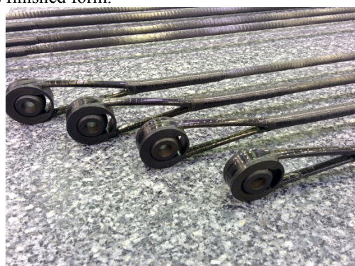
Figure 4: Carbon fibre cable manufactured by continuously wound tows of carbon fibre and consolidated with epoxy. Uniball end fitting are made of PBI engineering plastic.
