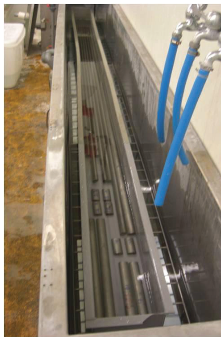
Figure 1: Stainless steel elliptical tube cleaning.
