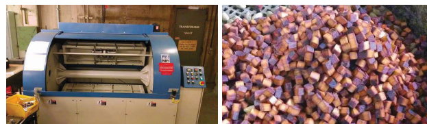
Figure 3: Centrifugal barrel polish machine loaded with Nb_3Sn cavity (left); and polishing media after 4.5 hours (right).
