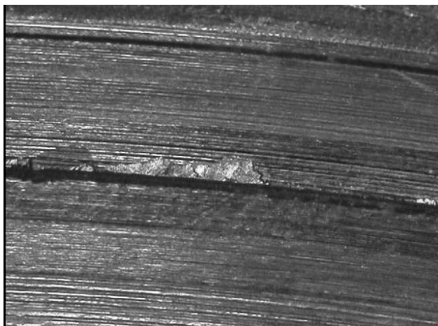
Figure 7: Microscopic picture of the knife edge of the hardened Nb1Zr flanges.
