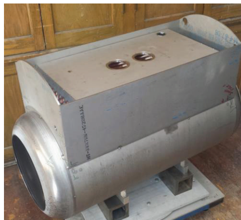
Figure 9: Helium vessel with superfluid heat exchanger.
