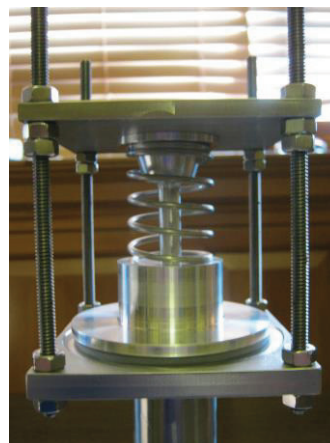
Figure 2: Prototype of the cryogenic safety valve.
